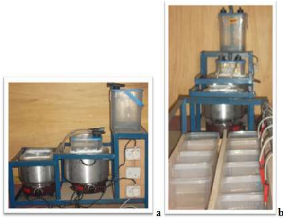
Plate 2: (a) Pictorial front views of activation bath, EN plating bath, replenishing tank (Ajibola et al. , 2014b; Ajibola et al. , 2015c) and (b) complete assembly of EN plating Bath (Ajibola et al. , 2014b, 2015c)
